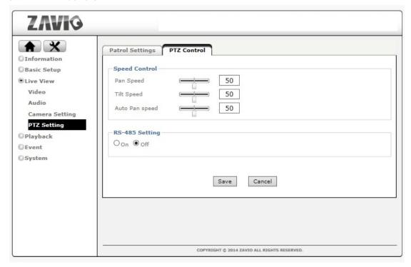
**Speed Control:** With higher speed, the camera would move faster.
